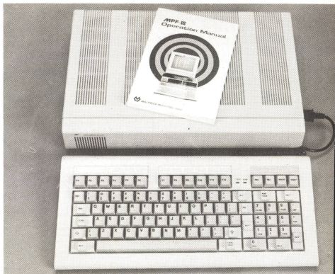
The MPF-III provides Apple II compatibility in a compact, low profile design with detachable keyboard. Features include an 80-column display, 64K RAM, printer and cassette ports and an Apple compatible hardware expansion slot. As yet however, no colour graphics are available. The February 1984 issue of Electronics Australia has a review of the system.
