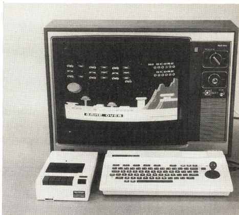
The Spectravideo SV-318 offers colour graphics and sound effects and a built-in joystick for $399. The graphics mode features 32 "sprites" or patterns which can be defined and moved around the screen independently of the remainder of the display, easing the task of writing fast-moving games and other display programs. The larger SV-328 does not have the built-in joystick but offers a larger, full-stroke keyboard. See EA for February 1984 for a review of the SV-318.
